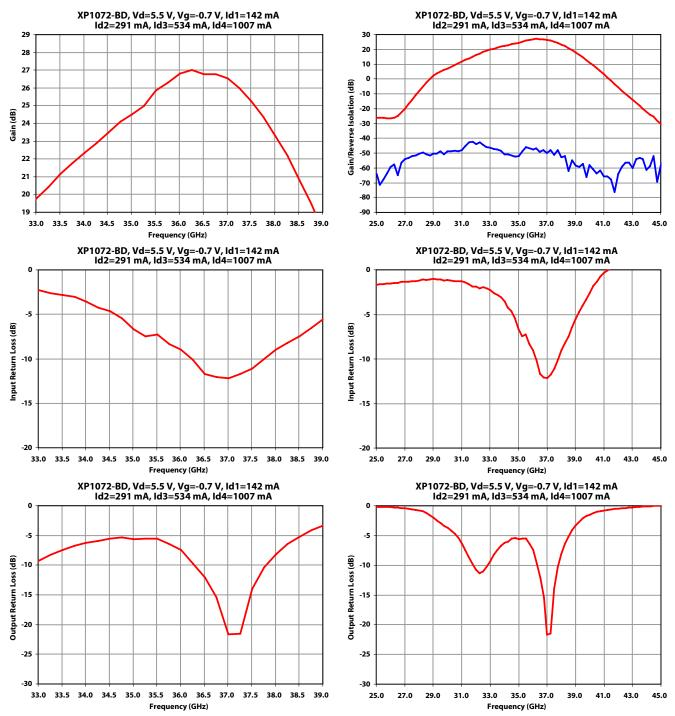
Note [1] Measurements – On-Wafer S-Parameters have been taken using reduced bias conditions as shown. Measurements are referenced 150 um in from RF In/Out pad edge. For optimum performance Mimix T-pad transition and tuned output matching network is recommended. For additional information see the Mimix "T-Pad Transition" application note. Contact technical sales for output matching network information.
