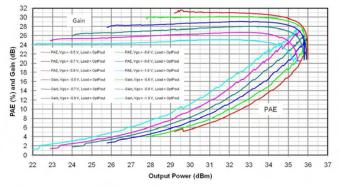
Note [1] Measurements – On-Wafer Gain and Output Power data has been taken using bias conditions as shown and 8us pulse width, 2.5 KHz pulse repitition frequency. Measurements are referenced 150 um in from RF In/Out pad edge. For optimum performance Mimix T-pad transition and tuned output matching network is recommended. For additional information see the Mimix "T-Pad Transition" application note. Contact technical sales for output matching network information.
